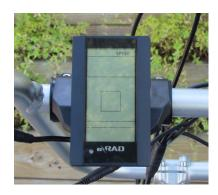
Step 16. Place console on LEFT side of handlebar crossbar as shown — using the spacers. If you don't put it to the left, the wires won't reach.
