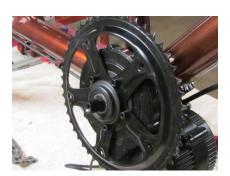
Step 20. Install chain guard with supplied bolts.
