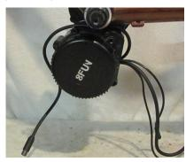
Step 11. Put the Y shaped bracket over motor shaft and insert two bolts through bracket and into motor. Do not tighten yet. NOTE: The Y bracket has bumps on one side. They MUST be on the inside, toward the frame, to lock it into place.
