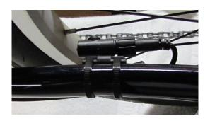
Step 25. Attach speed sensor magnet to a left side spoke so it passes just by the sensor.
