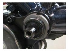
Step 12. Install gray lock ring over shaft, and tighten with supplied socket. Make sure it is very tight.
