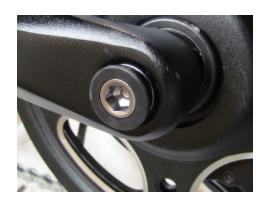
Step 21. Install new cranks and use new crank bolts. Securely tighten.
