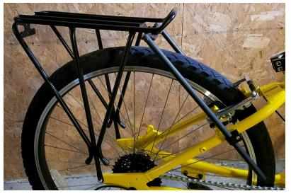
Step 4. Level rack and tighten all bolts.
