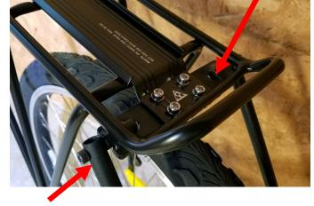
**Step 3.** Attach extension tubes to outside of custom mounting bracket with bolt. Attach bottom of tubes to threaded insert on seat stays using C clamp.
